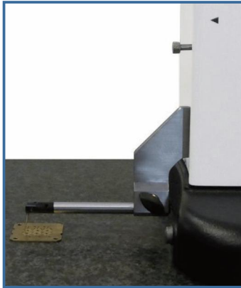
Watch movement height measurement
