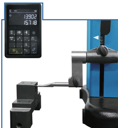
Diameter Measurement (Radius/Diameter Display Simultaneously)
