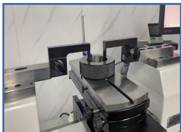
Smooth ring gauge for calibration
