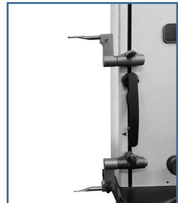
Adjustable measuring range
